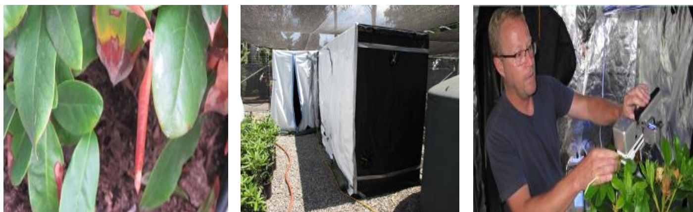
Figure 5: Photo of P. ramorum symptoms on rhododendron foliage (left photo), enclosed shelters for fluorescence measurements (center photo) and collecting fluorescence measurements inside the shelter (right photo).
